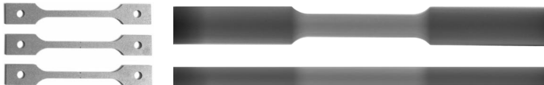
Images represent the tested specimens and the imaging from the computed tomography data for YZ and XY section planes at 60µm resolution.
