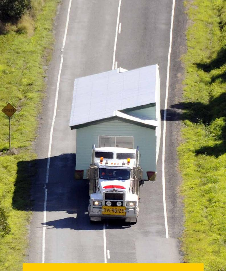
"Modular homes are constructed in our factory in Warwick QLD, transported to site in separate modules and finished off onsite. The largest home we've done had over 6 modules and including verandahs was over 700m2 in size!"
