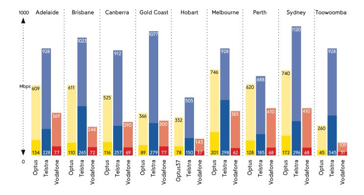
The graph shows the average throughput (darker shade) and the maximum throughput (lighter shade) for all technologies. All data sequences from the umlaut use case are taken into account.
