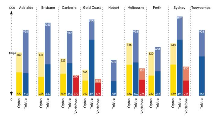
The graph shows the average throughput (darker shade) and the maximum throughput (lighter shade) for 5G only. All data sequences from the umlaut use case are taken into account. For Optus and Vodafone there are no 5G captures during the drive test in Hobart and Toowoomba.
