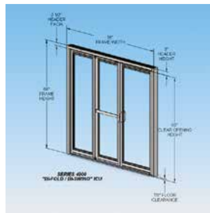
4900 series ALL-IN-ONE doors have overhead concealed manual door closers with a hold open feature
