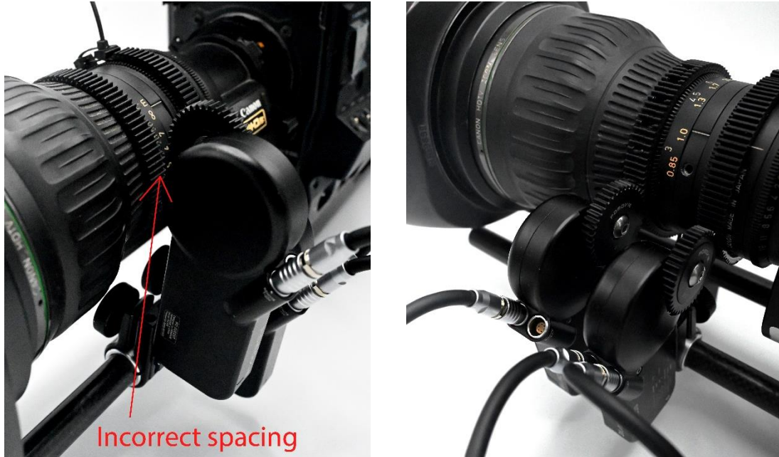
Figure 22: Incorrect and correct lens motor alignment
