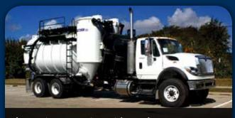
Ultra-quiet operation without the expense or weight of a shroud Advancements in blower and silencer technology eliminate the need for a sound shroud. The new shroud-free NX is priced right and the lower overall weight improves fuel economy, too.
