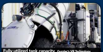
Fully utilized tank capacity Guzzler's VR Technology keeps the baghouses clean so the airflow remains strong throughout the vacuuming process. This enables the debris tank to be more fully loaded than conventional trucks before stopping to
