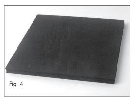
Care must be taken to ensure gaskets are installed right side up. The **flat** side of the gasket with the chamfered corners goes in the gasket retention groove on the door. Clean the gasket retention groove and use  $3M^{\text{TM}}$  yellow weather strip adhesive according to  $3M^{\text{TM}}$  instructions.
