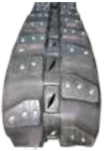
Rubber tracks with anti-spark teeth
