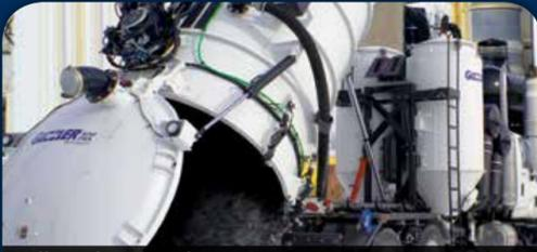
**Fully utilized tank capacity** Guzzler's VR Technology keeps the baghouses clean so the airflow remains strong throughout the vacuuming process. This enables the debris tank to be more fully loaded than conventional trucks before stopping to dump material. The fully opening door and 50° dump angle ensures quick unloading of the 18 yd<sup>3</sup> debris tank.
