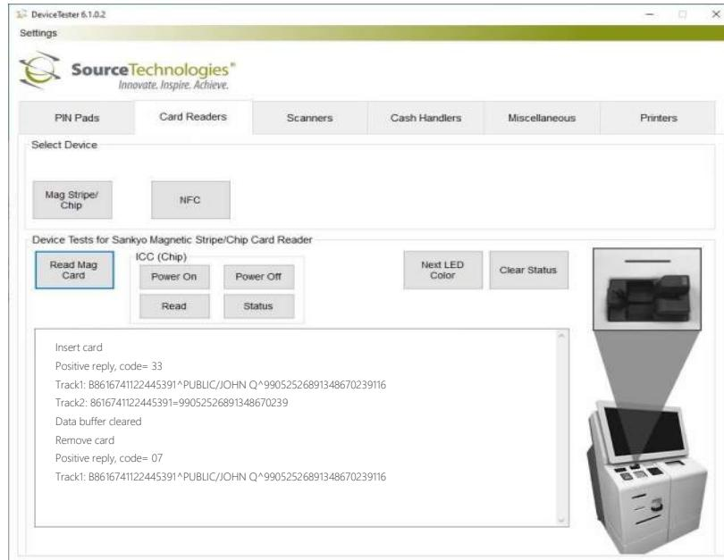
3. Tap the **Power On** button under **ICC(Chip)**. Insert card with a chip (NOT INCLUDED IN ACCESSORY KIT) and tap **Read** button.
