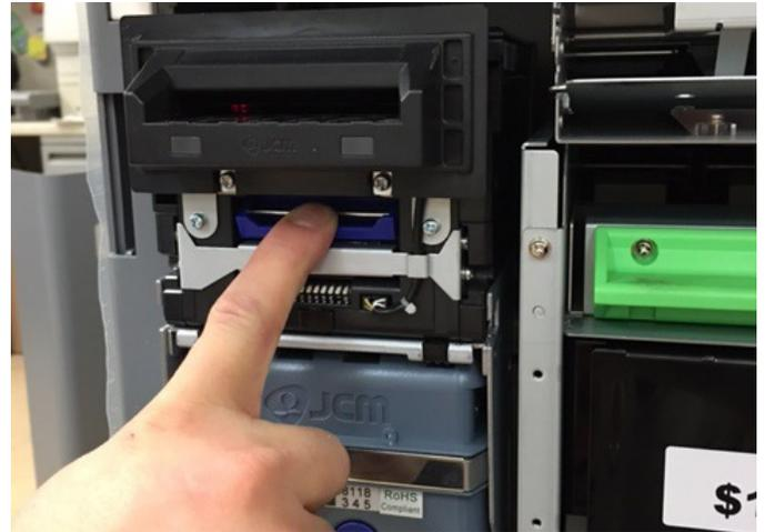
2. Firmly press the blue head mechanism lever down and pull the entire head mechanism out of the Cash Acceptor.
