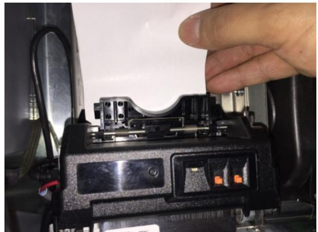
5. Hold the paper in this position for a couple of seconds until the printer begins to auto-load the paper.
