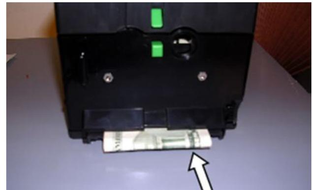
4. Push and hold the small green button on the front of the cassette to release the lock.
