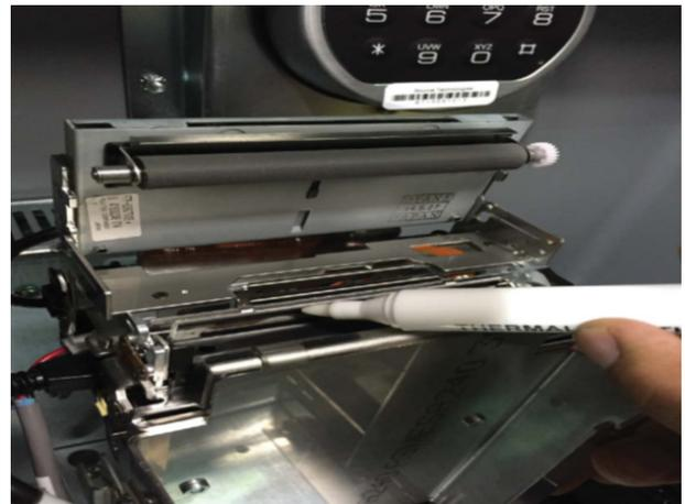
6. Rotate the printer mechanism downward until the mechanism locks.
