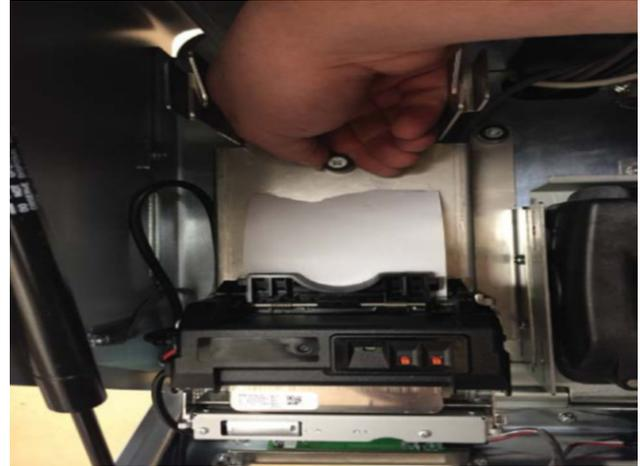
5. Using a thermal printer cleaning pen, wipe the pen's tip across the entire thermal head area.
