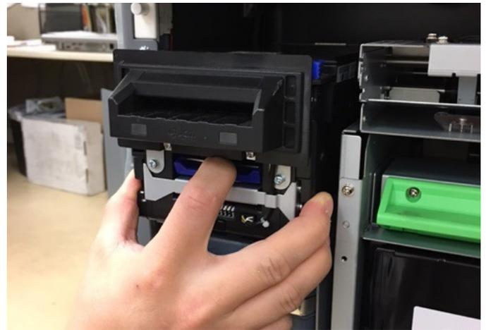
3. Clear Back Jams- Pull the top transport lever and open the transport cover to clear any jams.
