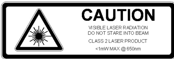
The optional laser barcode reader employed in this kiosk complies with US CFR1040.10 and 1040.11 except for deviations pursuant to Laser Notice No. 50 dated June 24, 2007, and EN60825-1:1994+A1:2002+A2:2001 and IEC60825-1:1993+A1:1997+A2:2001. The laser classification is marked on one of the labels on or near the laser device.
