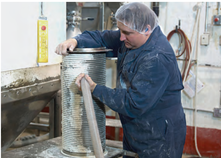
Quick cleaning: Operator opens end plate, removes basket, and cleans basket and sifter interior in 10 minutes.
