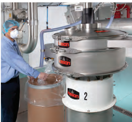
Downstream of the spray dryer, a Kason screener removes oversize particles. Because of the company's expertise in spray drying, "overs" (spout at right) comprise a small percentage of the total batch.
