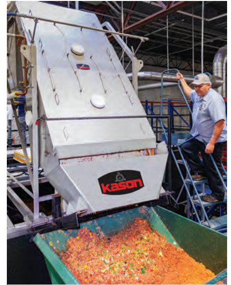
Wastewater flows over an inclined screening deck that captures peelings, stems, foreign objects and debris as small as seeds.
