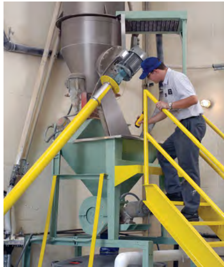
Operator checks flow of durum granular flour and recycled ground pasta into feed hopper, rotary airlock and 48 in. (122 cm) screener below.
