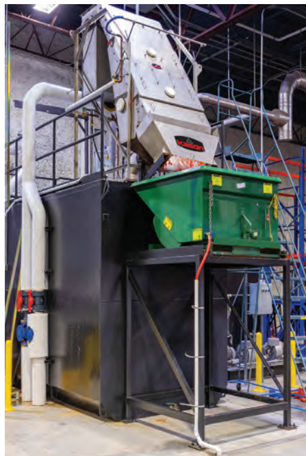
CROSS-FLO Sieve removes solids from 28,000 gal (106,000 l) per day of TGD Cuts' wastewater before it enters the municipal wastewater system.
