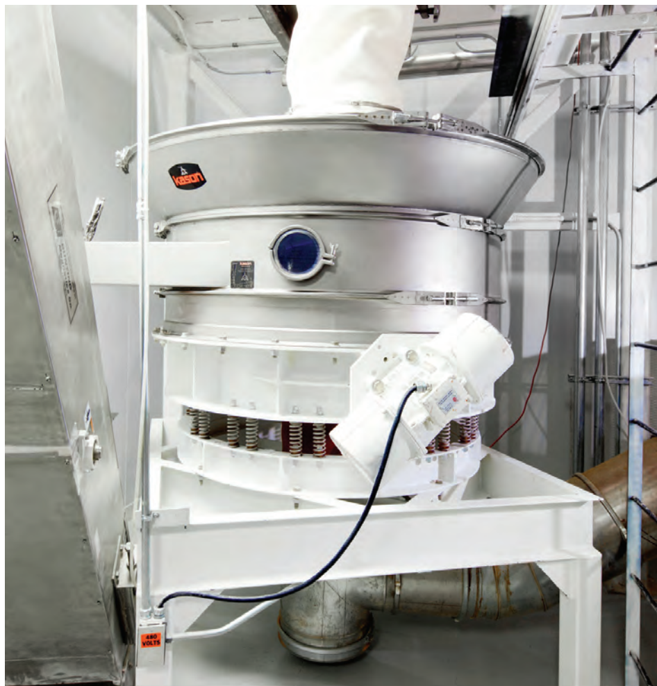
Powder enters the circular fluid bed processor through the top port. From the bottom, hot air is continuously blown upward through an enclosed circular screen on which the particles separate and fluidize. At timed intervals, liquids are added to the air stream to moisturize and agglomerate the particles, while the hot air continues to dry the material.
