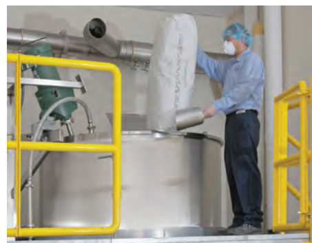
In the mixing room, an operator empties ingredients into the batching tank according to the customer's recipe.
