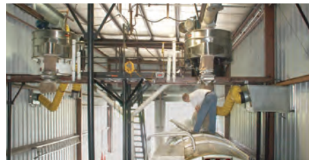
Two 60 in. (1524 mm) diameter Kason VIBROSCREEN screeners are used to load trucks with sugar at the SBS Sparta facility.
