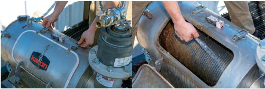
The sifter cleans easily as the front access door (left) opens for internal components to slide from a cantilevered shaft. The top access port permits quick rinse of the screen.
