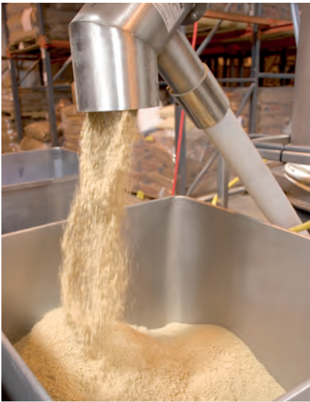
Screened dry ingredients are conveyed into a mobile bin that is wheeled to the processing side of the plant
