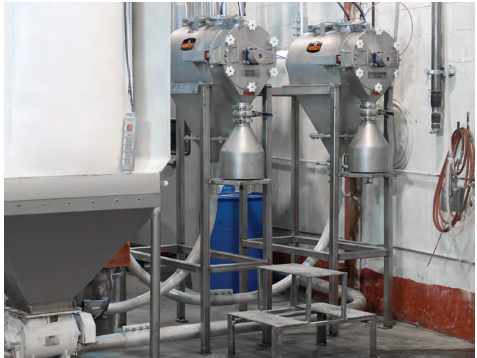
One pressurized CENTRI-SIFTER centrifugal sifter is dedicated to screening of white flour, the other for screening of whole wheat flour.
