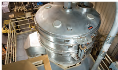
An 84 in. (2125 mm) diameter circular fluid bed cooler reduces the temperature of almonds with air cooled to 65°F (18.3°C) or less in one minute.
