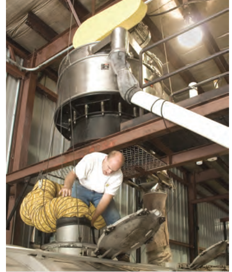
Each of the high-capacity discharge VIBROSCREEN units can screen up to 36 tons/hr, allowing trucks to be rapidly loaded with sugar.
