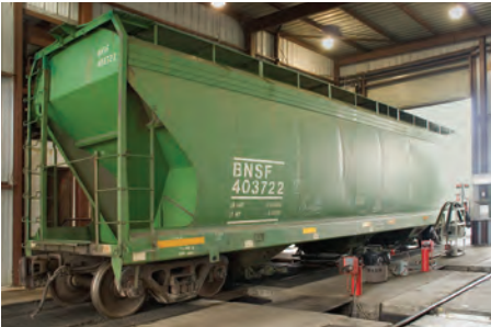
SBS Sparta receives dry-bulk granular sugars in covered hopper railcars.
