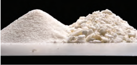
The facility's VIBROSCREEN screeners separate sugar lumps (right) from grains
