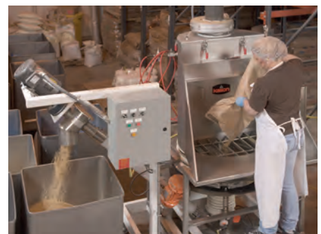
Mobile 30 in. (762 mm) diameter vibratory bag dump screener sifts dry ingredients prior to mixing them with meat protein. The waist-high unit minimizes physical effort in bag dumping, and includes a built-in dust collector.
