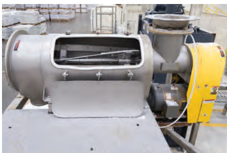
Rotating helical paddles create centrifugal force that accelerates on-size material through the screen, while propelling oversize particles through the downstream end of the screen cylinder. Nylon brushes affixed to the paddles prevent screen blinding.
