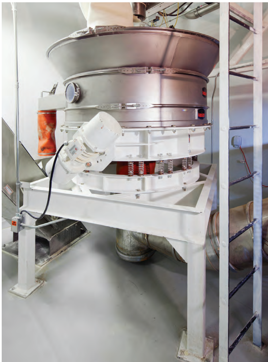
The circular fluid bed processor consumes significantly less floor space than the rectangular fluid bed dryer originally considered.
