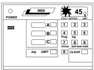
Press the '6' key. The display will show a 4-digit 'Control Code' as two pairs of numbers, e.g. '45' then '68'. The 'Control Code' will be displayed 7 times, write down code.
