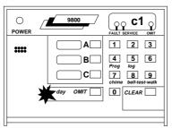
Any circuits which are open will be displayed in sequence. If no circuits are open the display will show "-- --".
