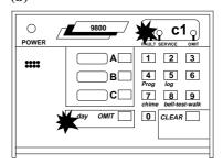
The instruction which first caused the alarm condition will be displayed. The 'Fault' LED will also be be illuminated.
