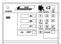
Go to a system keypad, then keyin your valid access code. The display will show the circuit which first caused the alarm, plus the 'Fault' and 'Service' lights. **(b)**
