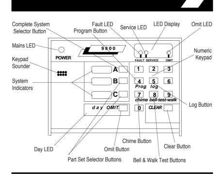
Setting, unsetting and access to the system functions are normally inhibited unless a four digit security code is entered via the remote keypad.
