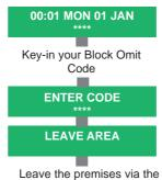
Leave the premises via the prescribed exit route. The system will automatically re-arm the circuits in Group 'D' on expiry of the exit timer or closing of the final door, or pressing the exit terminate button.
