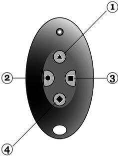
The 722r, 723r, 727r and 728r telecommands have four buttons that you may program for separate functions.
