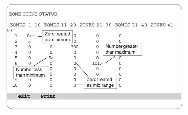
You can print this "Zone Count Status" using the **Print** function on the Function Bar.
