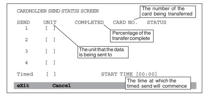
Data can be sent immediately or the Cardax Commander can be set to send the data at a given time. With a number of new units are added to the system and a large amount of data, a transfer can take a considerable amount of time (10,000 names to 50 units takes about 3 hours).
