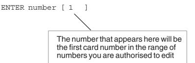
At this point you are asking the Cardax Commander to find the first free card number after the one that you have specified. If you wished to have a range of card numbers that were exclusive to one department (for instance) you could create cards from 1,000 onwards by entering 01000 at the previous prompt. The Cardax Commander would then find the next free card number after 1,000.
