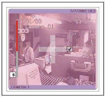
This screen overlays the current playback video and allows the user to enable or disable motion detection on the screen within blocks that form a  $16 \times 16$  grid.
