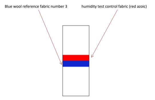
Put prepared card into the specimen holder and cover with a  $\frac{1}{2}$  mask:
