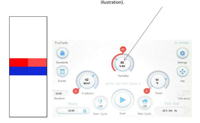
If the humidity test control fabric (red azoic) has faded less than the blue wool then the effective humidity is too low& so needs increasing on the dial (illustration only).
