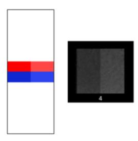
It is very likely that this will not happen on the first test fade and the humidity test control fabric (red azoic) will either be faded more or less than the blue wool reference fabric. If this occurs, then you will have change the RH% on the dial to do a new test.
