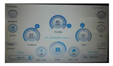
6. If you choose use the Black Panel Thermometer BPT and not the Black Panel Thermometer BST Solarsens as advised, then it is necessary to try and control this through setting the chamber temperature at initially approximately five degrees lower than the BPT listed in ISO 105 clause 7 Table 2 (it gives 40+/-3°C).
