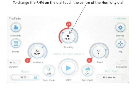
The numeric keyboard will appear - type in the humidity level you think you will need (remember this is trial and error & the amount you increase or decrease the RH% number by depends upon how different the fade steps are between the humidity test control fabric (red azoic) and the blue wool fabric fades when compared to each other).
