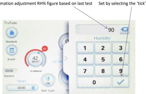
Estimation adjustment RH% figure based on last test
