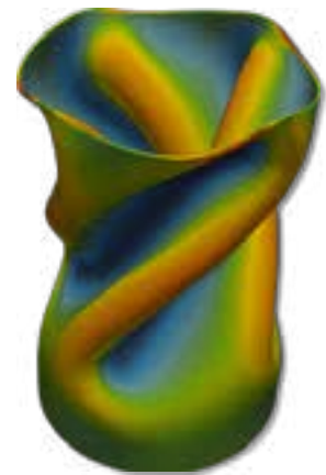
Plastic torsional buckling of a thin-walled tube
