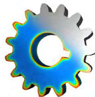
Surface heat treatment (carburizing, quenching, tempering)
