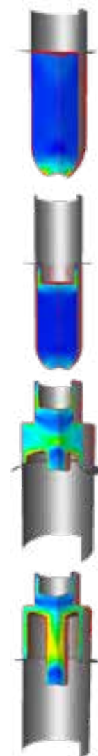
Cold forming a valve cage on an automatic transfer press
