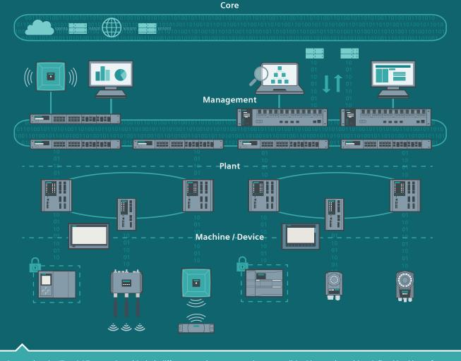
Connecting the IT and OT networks, with their different requirements, can be accomplished by starting with a defined backbone for the industrial side. The machine and plant-floor aggregation levels are in production scope. The backbone aggregation level is still an integral part of the production scope but aligned with IT in regard to the interface.
