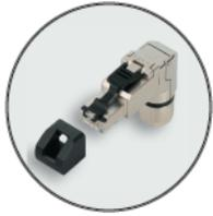
LUTZE's RJ45 connectors are designed with a rugged zinc die-cast metal housing with quick-connect IDC (Insulation Displacement Connector) technology that is user friendly with labor and time saving features as no special tools are required, making them ideal for quick field wiring in industrial applications.
