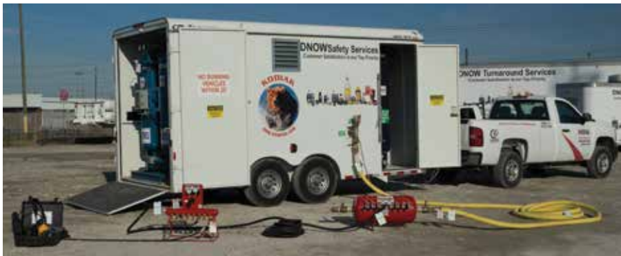
Kodiak low-pressure compressor trailer
