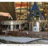
Valve is flushed, cleaned and inspected
