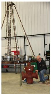
Damaged parts are discarded and replaced, all soft goods are replaced
