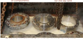
Metal parts are stripped of any petroleum products and paint
