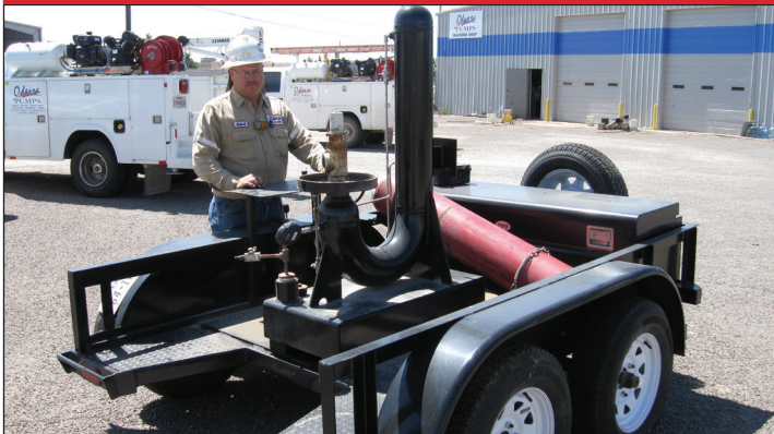
RELIEF VALVE TESTING
