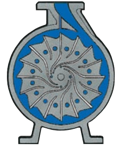
Circular concentric casing
