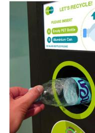
The machine can accept any container or only those within a database. The database can be uploaded digitally or be set up manually, which is recommended if a small range of containers has to be accepted.
