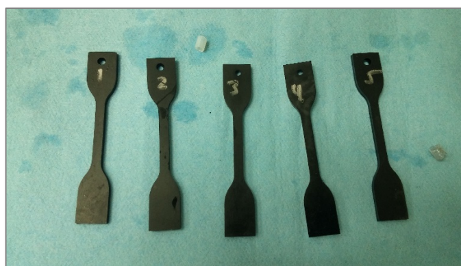
Figure 1: Gazguard 728 samples after 160 hrs immersion in sour gas and Jet Fuel A multiphase mixture
