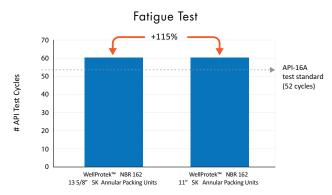
\*\*FO&GT fatigue test stopped at 60 cycles. Units were not taken to failure.
