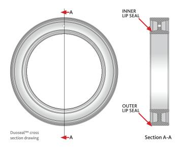
The Vector Duoseal™ is proven in sizes from 2" to 34" in water depths up to 13,125ft (4,000m) at temperatures ranging from -50°C to 150°C, and at pressures up to 15,000psi, making it suitable for most known subsea applications, and as an alternative to RIT rings for Topside joint integrity.
