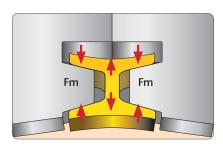
NOTES: The self energization force is a fraction of seal geometry and is never sufficient to indent the hub faces.
