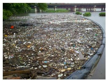
The Lamor Solid Floatation Boom (SFB) has been developed to meet today's requirement for a quick to deploy and economical containment boom system.
