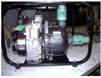
All internal and external fasteners are stainless steel. Buna-N, EPDM or Viton elastomers are available from stock. As pictured above, the Pacer Pedestal Pump is coupled to either a plastic pedestal with carbon steel shaft or a cast iron pedestal with stainless steel shaft.
