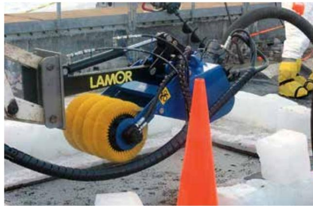
Lamor Recovery Bucket 400 (LRB 40), capacidad: 19 m<sup>3</sup>/h (83 gpm)
