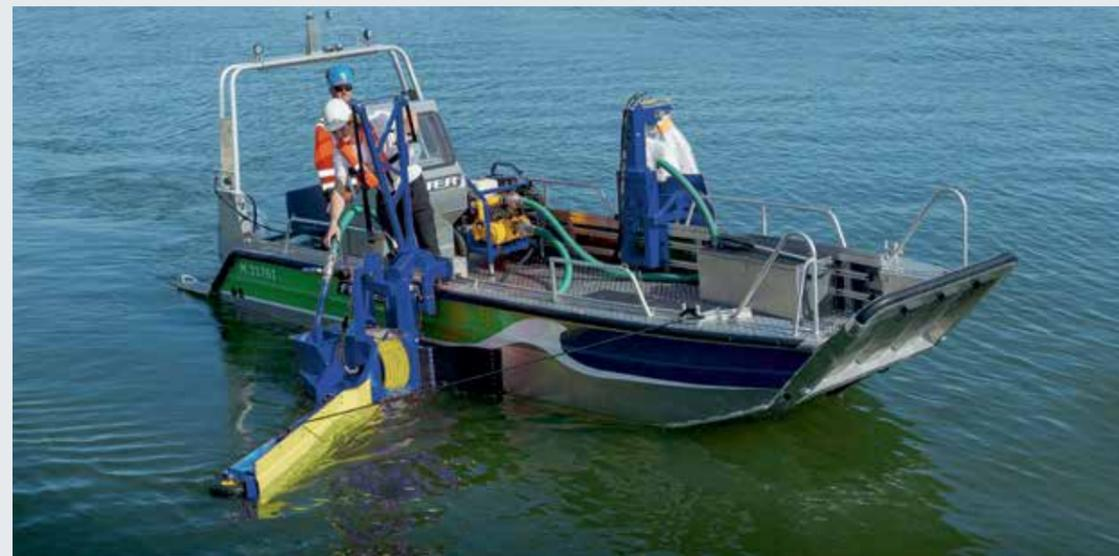
Colector lateral / MiniBagger, capacidad: 10 m<sup>3</sup>/h (44 gpm)
