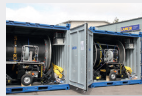
Containerized Solution for Heavy Duty Oil Boom HDB 1500
