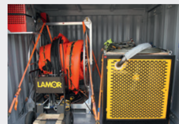
Containerized solution incl. power pack, hose reel and hydraulic control set for skimmers
