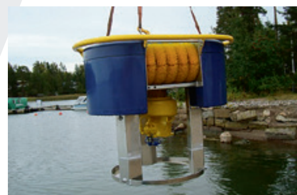
Multiskimmer (LMS 50/70), capacity: 271.5 m 3 /h (1,195 gpm)
