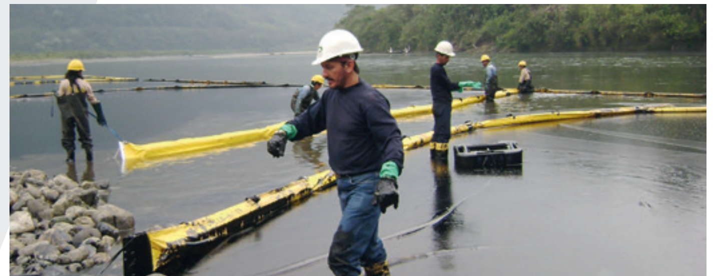
Solid Flotation Boom, height: 360-920 mm (14-36 in)
