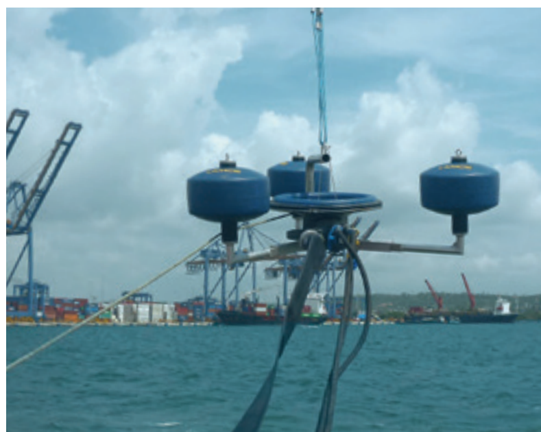
Weir Skimmer 800 (LWS 800), capacity: 112.2 m 3 /h (494 gpm)
