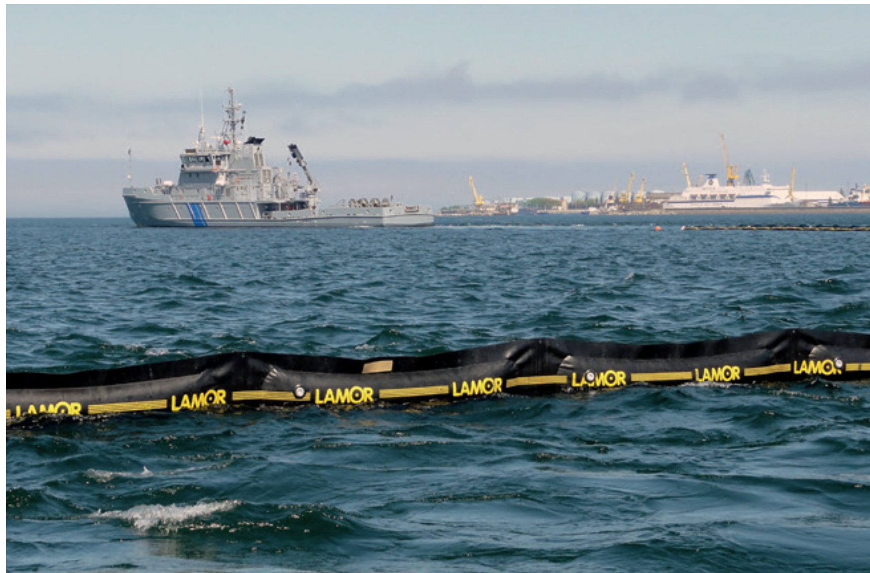
Heavy Duty Boom - (Rubber & Neoprene), height: 900-2000 mm (35-79 in)
