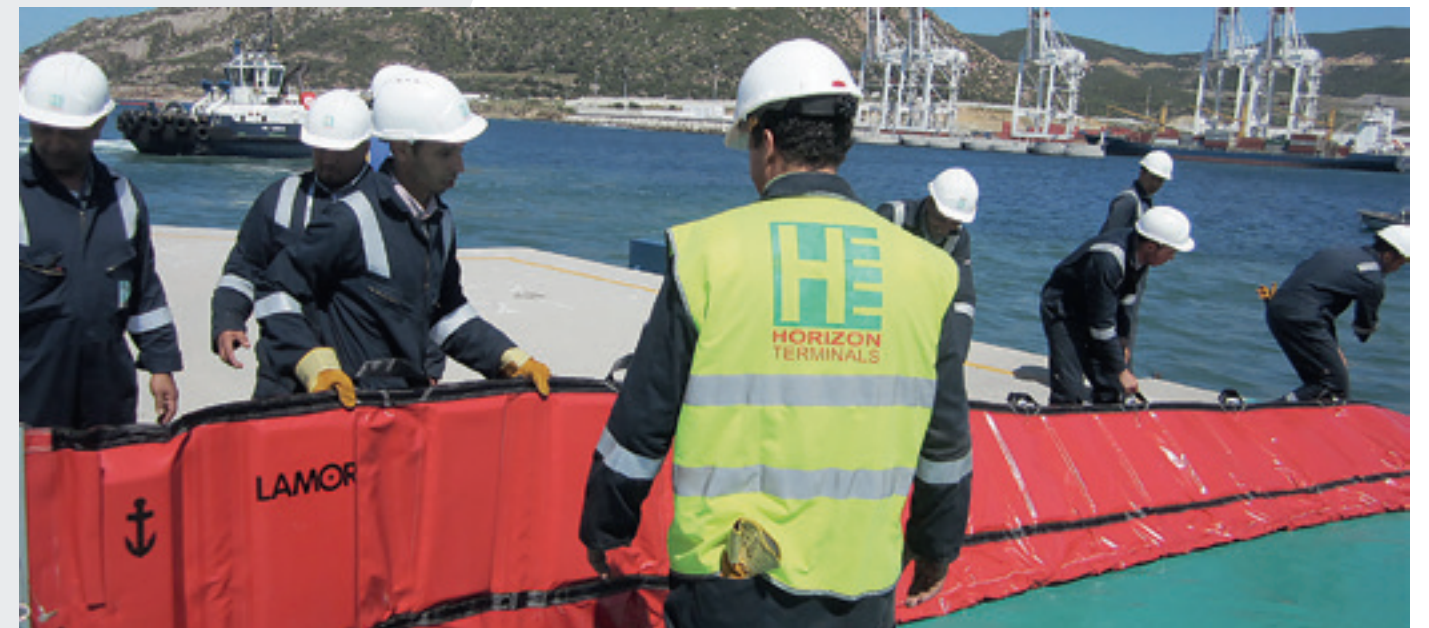
Foam Filled Boom, height: 350-1500 mm (14-59 in)
