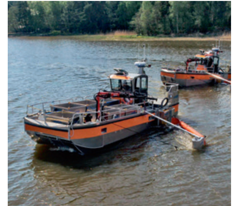
Ultra Shallow Draft Workboat equipped with side cassette for oil recovery
