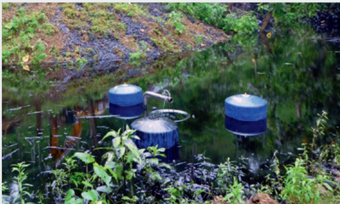
Weirskimmer 500, capacity: 70 m 3 /h (308 gpm)
