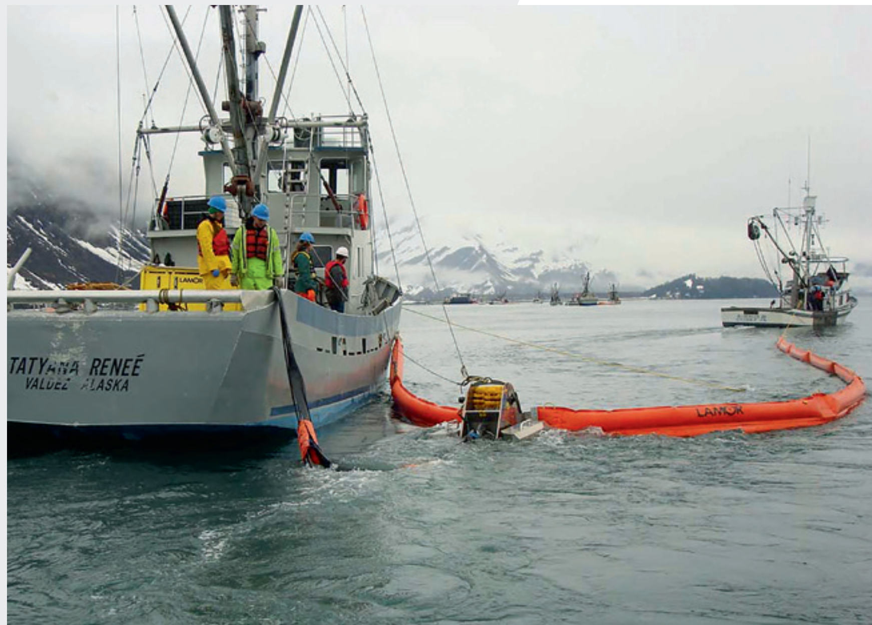
Multimax 50 (LAM 50), capacity: 50 m 3 /d (220 gpm)
