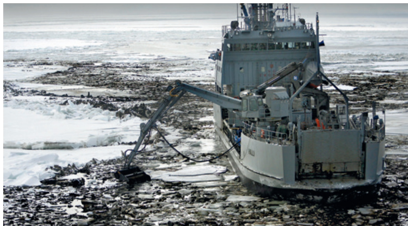
Bucket Skimmer (LRB 250), capacity: 140 m 3 /h (616 gpm)
