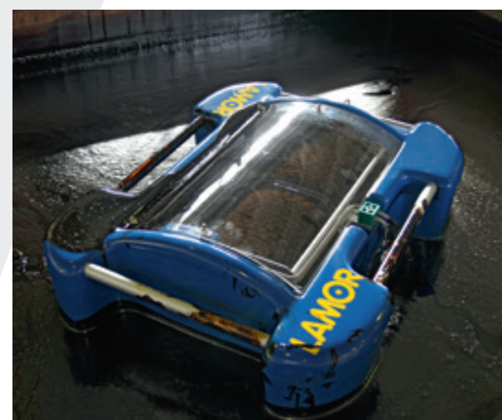
Minimax12 (MM12), capacity: 12 m 3 /h (52 gpm)
