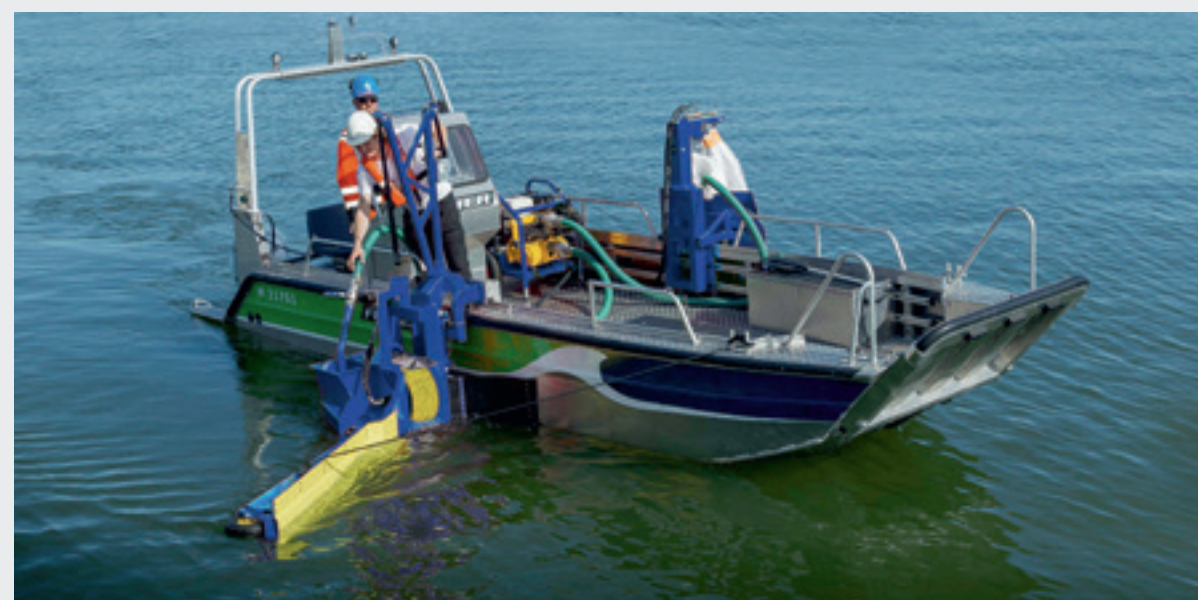
Side collector / MiniBagger, capacity: 10 m³/h (44 gpm)
