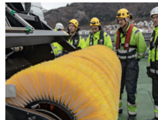
Vessel-mounted Bucket Skimmer (LRB 150), capacity: 115 m 3 /h (506 gpm)
