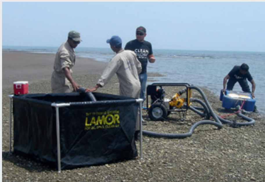
Collapsible oil storage tank, LPP 6 C 75 and Minimax 12 skimmer
