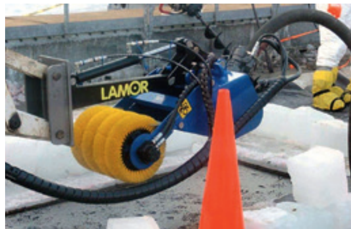
Lamor Recovery Bucket 40 (LRB 40), capacity: 19 m 3 /h (83 gpm)
