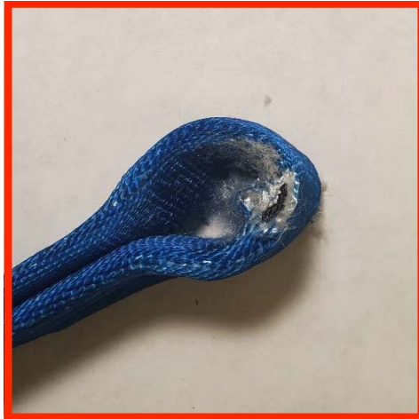
Unacceptable Levels of Wear
