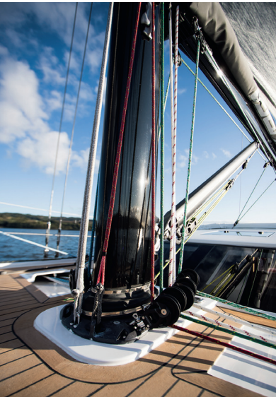
The design team wanted to avoid the mast piercing the coachroof. This leaves a large flush foredeck, which includes a sail locker and an anchor locker. The bowsprit neatly hides the anchor roller and all lines are led under
