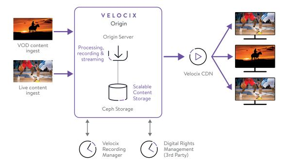
Velocix Recording Manager integrates seamlessly with Velocix Origin and Velocix CDN to provide an advanced time-shifted content delivery capability with software-defined storage for limitless capacity
