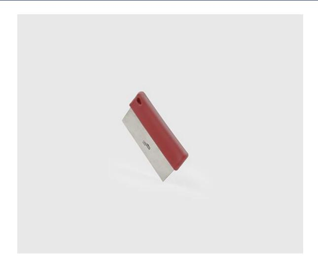
Dough cutter with coloured, slip resistant Polypropylene handle (maximum dimensions 162mm x 16mm), contoured for easier holding, and hanging hole. The stainless steel blade is 152mm wide, 45mm out and 1.4mm thick.
