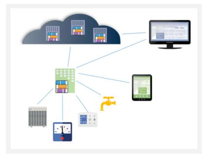
In this architecture, a node running SkySpark is installed in the facility and connected to local data sources via a variety of standard data acquisition connectors including: Bacnet IP, Modbus TCP, Obix, Haystack, SNMP, Sedona, OPC UA, SQL, and the REST API – all included with SkySpark.
