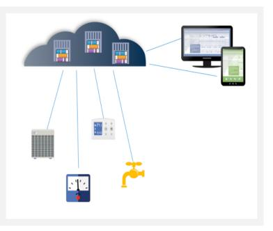
distributed over multiple servers for load balancing and performance optimization. "Live polling" of data from end devices is also supported in this architecture, but the application designer needs to consider the effects of network latency, bandwidth, communications faults and the ability of end systems to support the necessary volume of polling requests.
