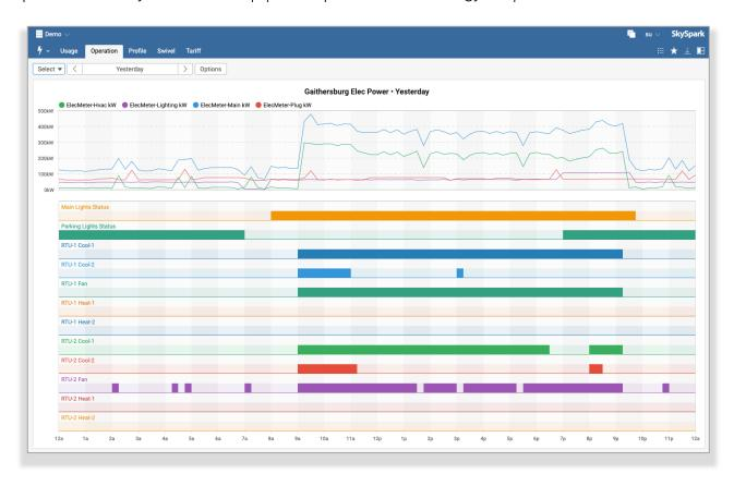
Above: The **Operations View** shows energy use (demand as shown) correlated with equipment operational status. This provides clear insight into the impact of equipment operation on energy use.
