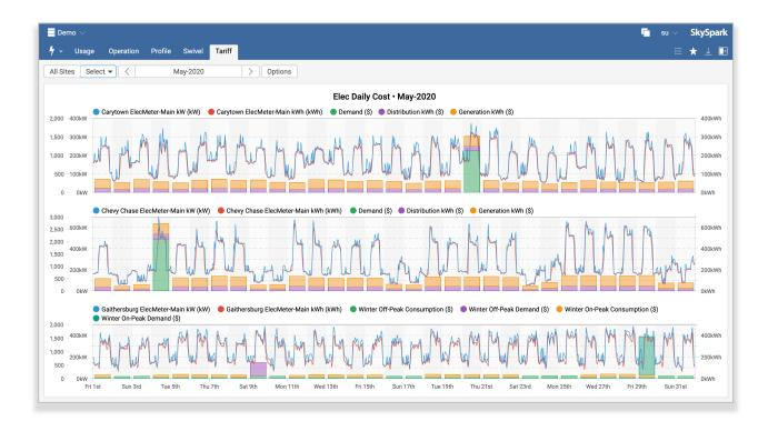
In the view above the line graphs represent the consumption and demand values from the meters. The vertical bar graphs represent the costs calculated based on the charges associated with the Tariff rate. SkySpark automatically correlates energy use and cost data and overlays them to provide operators with a clear view of how energy consumption and demand impact actual energy costs.
