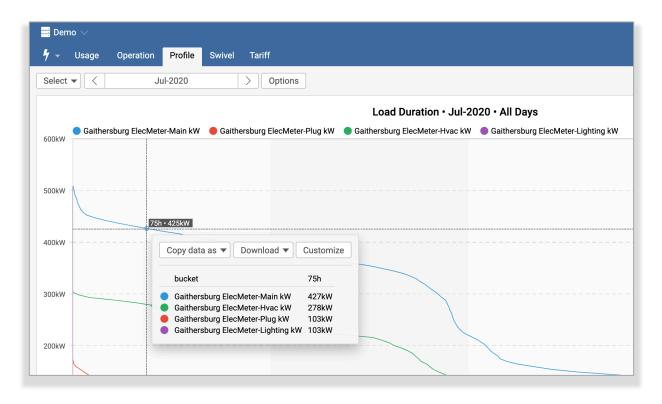
In the view above we can see that the Gaithersburg site Main kW meter exceeded 425 kW for 75 hours in the month of July.
