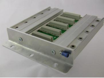
The kit is composed of 2 squares and 4 screws. The squares are fixed at the sides of the rack. The black plastic sides must first be removed as well as the GND screw. The latter must be screwed to the square after fixing.
