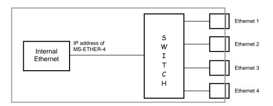
If you want to access the **TBox MS** from devices connected to the Ethernet, the devices you connect to the switch **must be in the same subnet** than the one of MS-ETHER-4 (correspondence in IP addresses and subnet mask).
