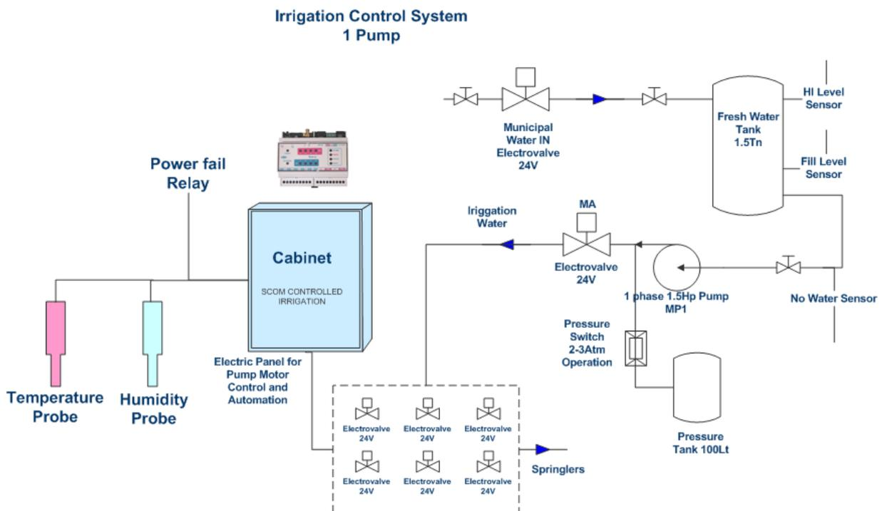
It is desired to setup and operate a simple irrigation system based on SCOM-100.
