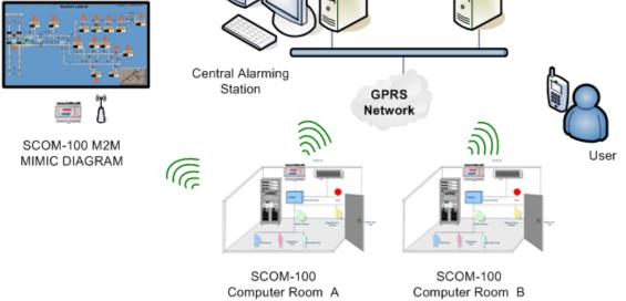
Infinite SCOM-100 is a GSM/GPRS Edge compatible cellular RTU solution designed specifically for remote monitoring of server rooms. Compared with traditional SNMP solutions, that require Ethernet presence, cellular offers a reliable way access server rooms, when the existing IT infrastructure has failed.
