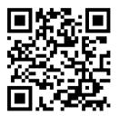
Print-and-cut jobs include an HP barcode as part of the print. This is read by the OPOS to find out where the cuts should be made. See <u>Read the HP barcode on page 24</u>.
