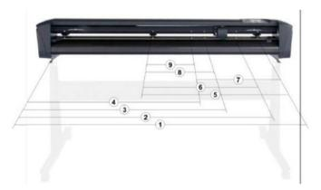
7. Position the pinch rollers over the drive sleeves about 3 to 15 mm (0.1 to 0.6 in) away from the substrate's outer edges (1). Then pull the substrate while holding the flange at the back, so that the substrate is tight.
