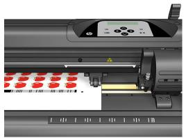
If there are different jobs on the same sheet or roll, with different justifications, the carriage should be placed as shown below.
